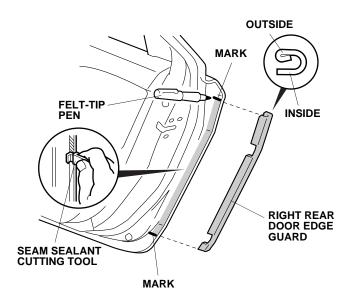
Position the cutting edge of the seam sealant cutting tool against the door edge, and trim the seam sealant from mark to mark.
