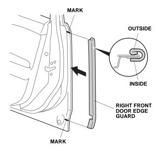
8. Using a rubber mallet, lightly tap around the bend in the right front door edge guard.
