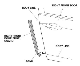
4. Using a felt-tip pen, mark the inside edge of the front door at the upper and lower ends of the right front door edge guard.
